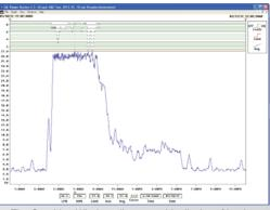
The Graphing Window allows graphic display of load profile and control information.
